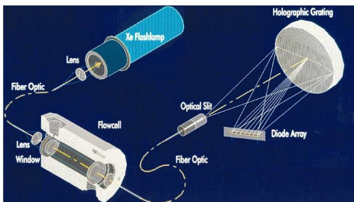
The instrument is composed of an UV lamp and a diode array. The UV beam, after passing through the measurement cell, reaches a holographic grating disk. This one diverts each wavelength composing the beam onto a specific diode of the array. The voltage emitted by the individual diodes is measured and this information is acquired by the embedded computer through a serial line.
