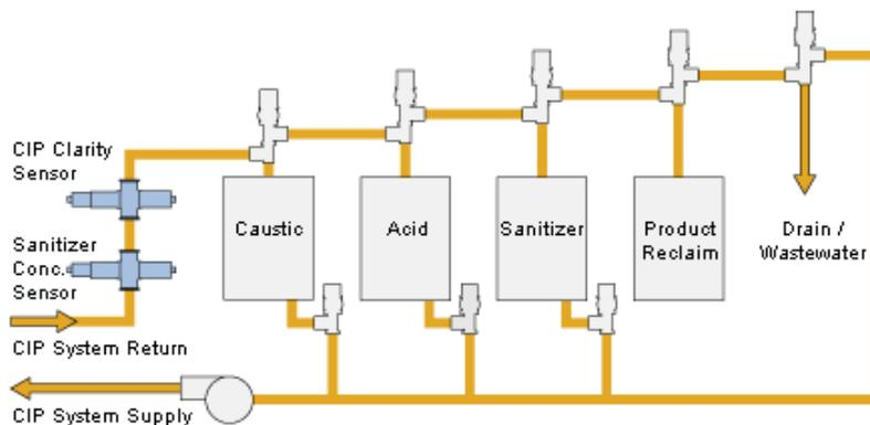
NOTE: according to the Customer's requirements, the PLC (embedded computer) can either control the whole CIP process or only the spectrophotometer.
