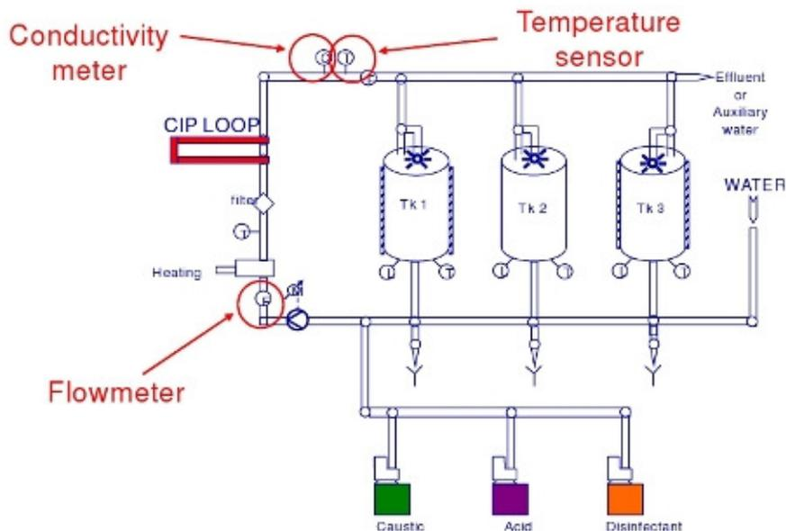
Since the various cleaning solutions are more conductive than the water used for flushing, conductivity measurement is a logical way to monitor the cleaning steps and the final rinse.
